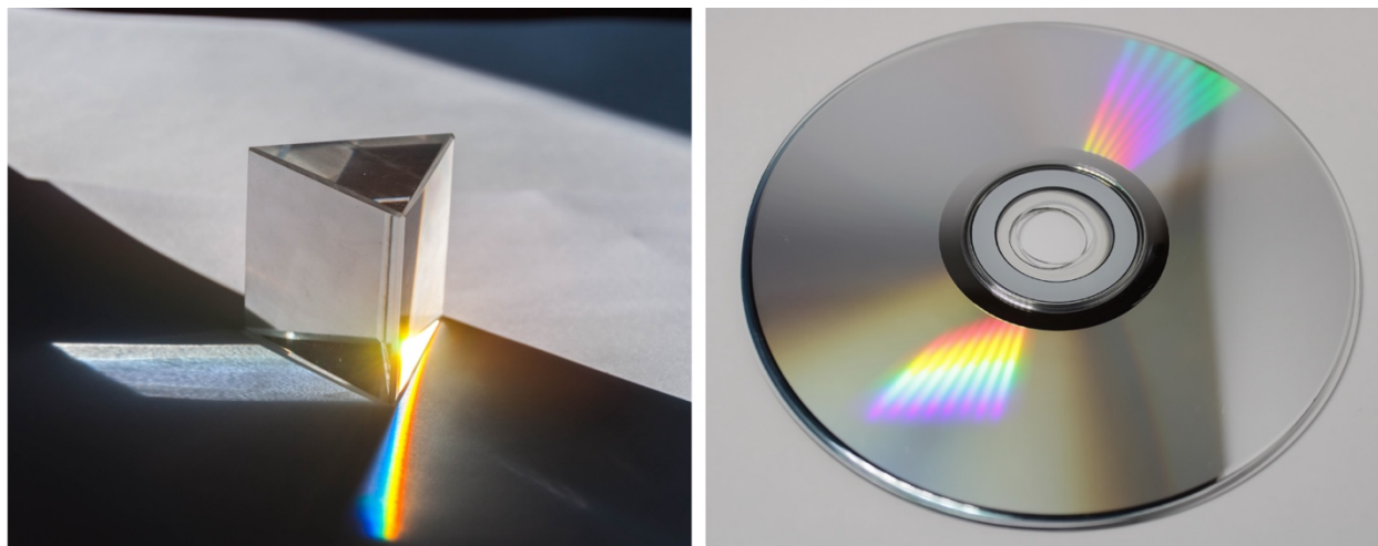
Figure 1. When sunlight passes through a prism, it bends and separates into its color constituents (left). The shiny surface of a DVD or compact disk (CD) also separates light into its components and reflects them back to your eyes.
