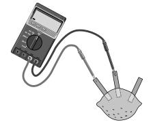
8. Set up a friendly competition among different student groups to design a battery that will give the highest voltage. Some questions to consider: (a) What combination of metals gives the highest voltage? (b) Does the voltage depend on the separation between the metals? (c) Can pairs of metals be connected in series to increase the voltage of a citrus battery? (d) Is the battery voltage stable over time? (e) How long will the battery last?
