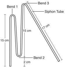
Figure 1. Self-starting Siphon Tube.
