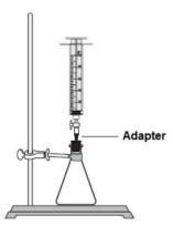
Figure 1. Gas collection apparatus.
