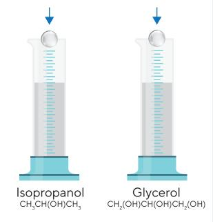
**3.** The marble dropped into the isopropanol-containing cylinder hits the bottom faster than the marble dropped into the glycerol-containing cylinder.
